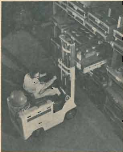
Surprising variety of fuel-cell-powered vehicles already have been designed, built, and tested by one of the major research groups active in American basic fuel-cell development. Clockwise from upper left, a one-man submarine, two-man golf cart, 2,000-lb-capacity lift truck, and earliest fuel-cell vehicle to be developed—a tractor with 3,000 lb of pull.
