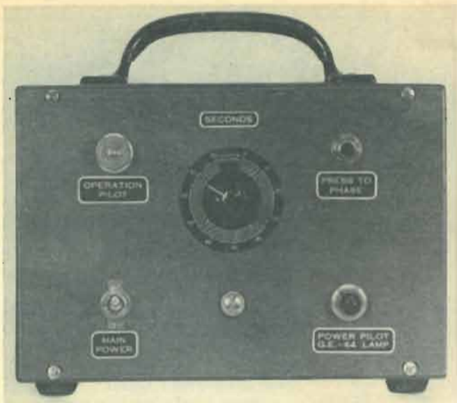
Neat labeling enhances front panel of the vacuum-tube timer. It's also a good idea to tag back-panel controls and switches.
