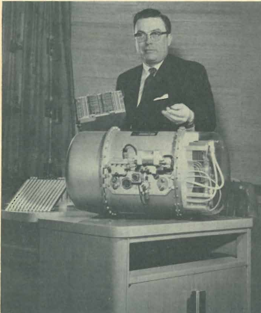
One of the Gemini fuel-cell units in fully encased form, as a single cell (at far left), and as a cell-stack module—one of three such modules making up the complete system.
